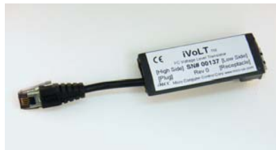
I 2 C Bus Voltage Level Translator (iVoLT)
