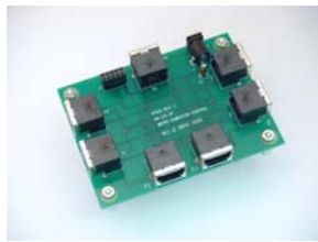
I 2 C Bus Distribution Board (IP-201)
