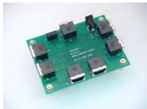
I 2 C Bus Distribution Board (IP-201)
