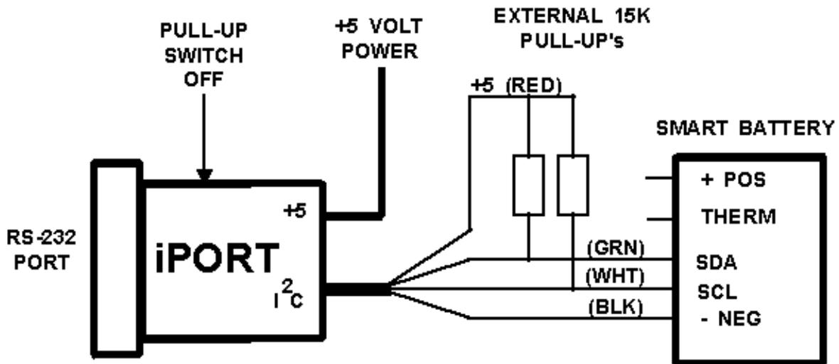
2. Connect iPort Host Adapter to target SMBus Smart Battery. (See suggested setup above)
