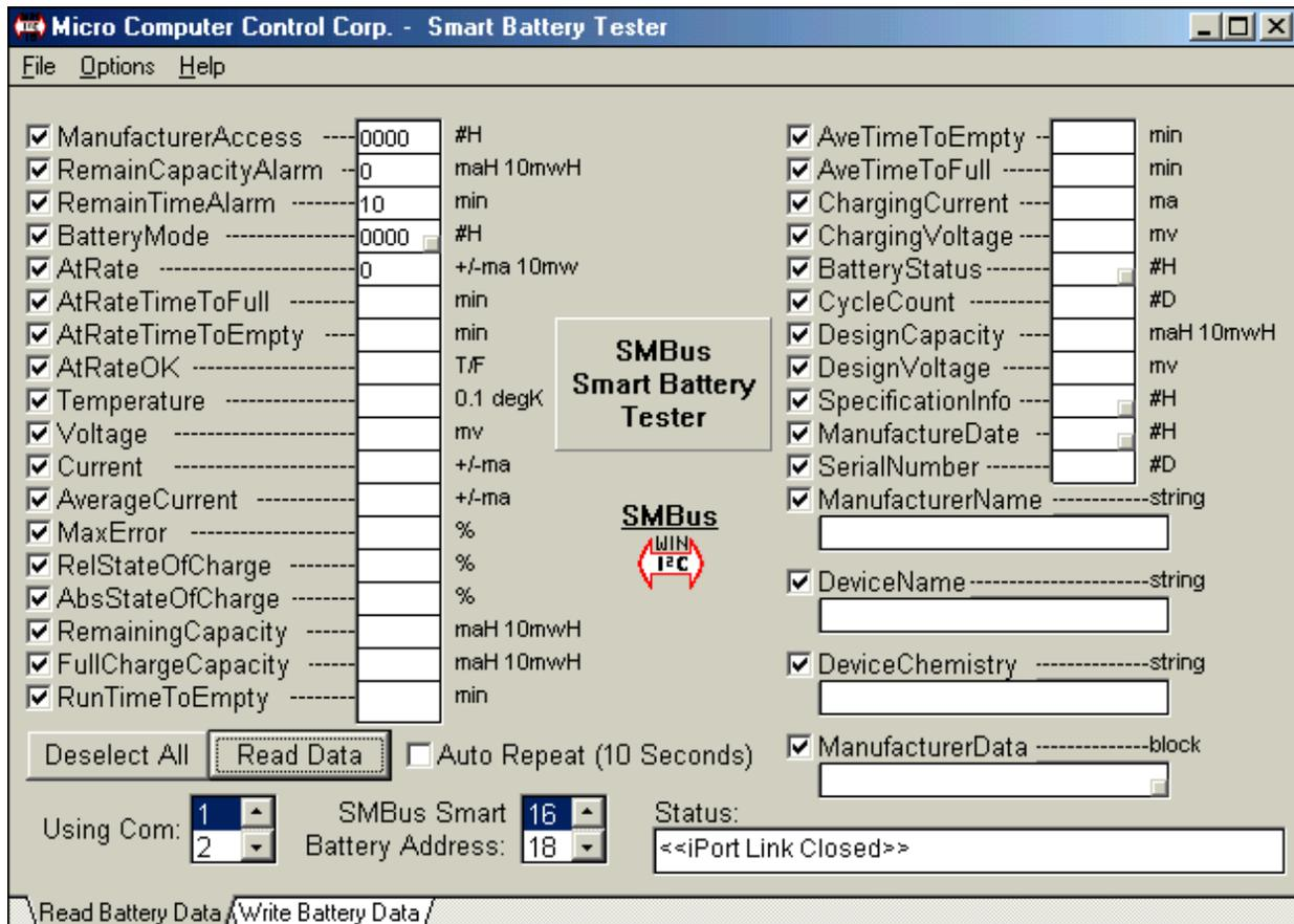
This document contains information on the MCC SMBus Smart Battery Tester Software including equipment setup and usage.
