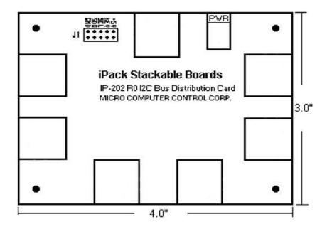
If the unit is powered from the power jack (J3), a +5VDC Wall Transformer (MCC Part# MWT-5VA) is required.
