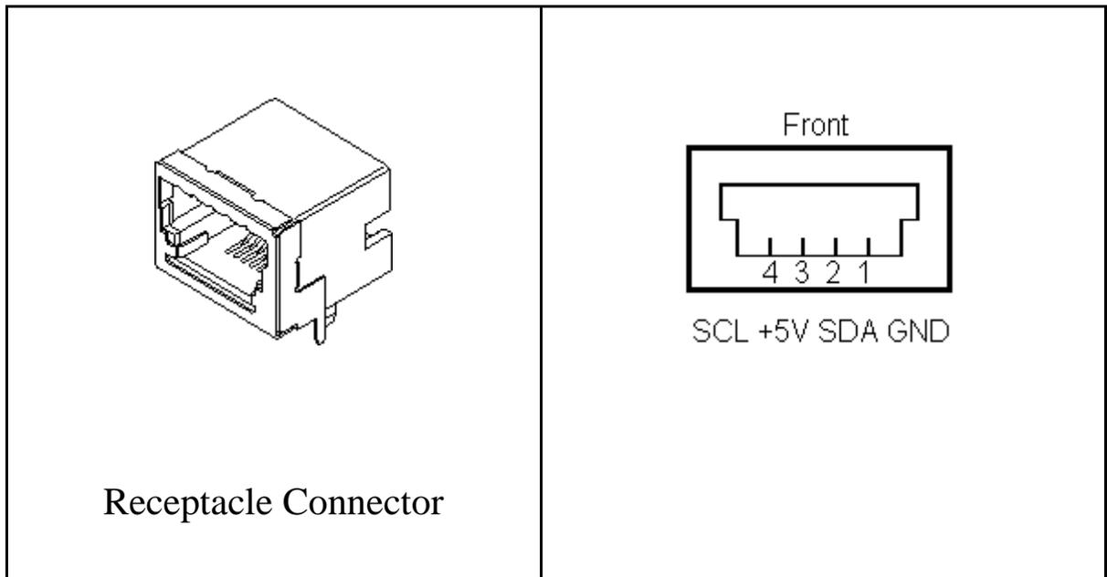
An I<sup>2</sup>C Interface Cable (White=SCL, Red=+5VDC, Green=SDA, Black=Ground) is provided to connect to an external I<sup>2</sup>C Bus. Since there is no standard I<sup>2</sup>C Bus connector, you may want to cut off one end of the cable and add a connector compatible with your target system.
