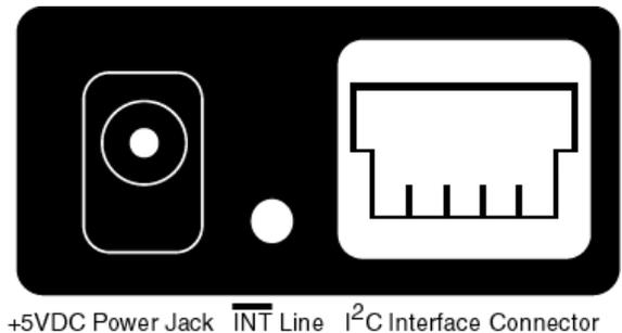
+5VDC Power Jack INT Line I<sup>2</sup>C Interface Connector
