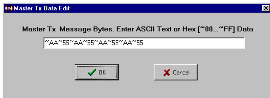
In the data editor, enter one or more ASCII text characters or hexadecimal data bytes. Each hexadecimal byte is entered as two ASCII-Hex characters (00 to FF) preceded by a tilde (~) character. ASCII text and hex data can be intermixed, as long as each hex byte is preceded by a tilde.
