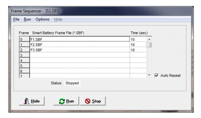
A Smart Battery Data Frame consists of set of Smart Battery Data values displayed on the emulator's main screen. These data values can be saved to a Frame file using the File|Save Frame menu on the main screen.
